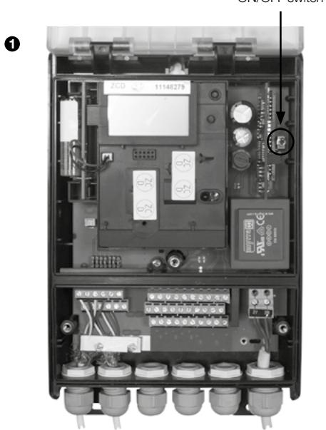
Install the configured Modbus card under the metrological block of the CF800, position option1
