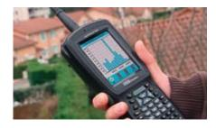
ACE Vision Mobile is an extension of ACE Vision available for HHU and laptops. This mobile software can be used for meters with or without modems, as a backup in case of standard communication media failure or during a maintenance session.
